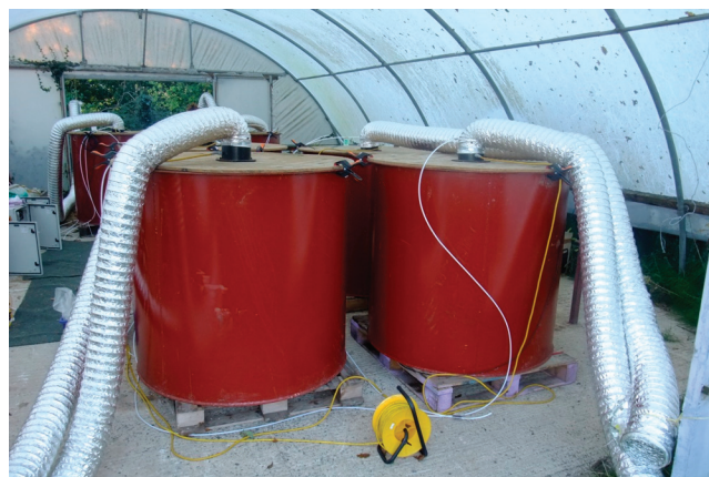
Fig. 1. Pilot-scale slurry storage tanks with specially adapted lids for gaseous emission measurements.
